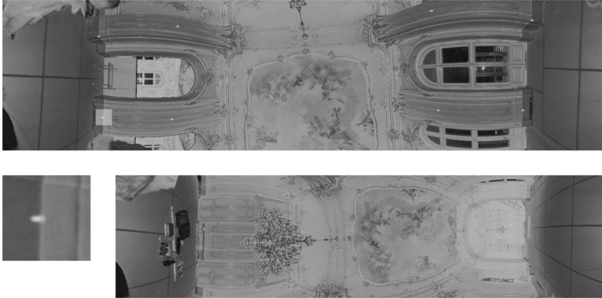
*Fig. 1:* The upper image shows a measurement across the longer axis of the room, the lower right image shows a measurement along it (each  $1800 \times 444$  single measurements). The lower left image depicts an enlargement of the marked area in the upper image. It shows an area of  $40 \times 40$  single measurements, conforming to an object size of  $60 \times 60 \text{cm}^2$ . (This projection is the Equirectangular projection by Marinus.)
